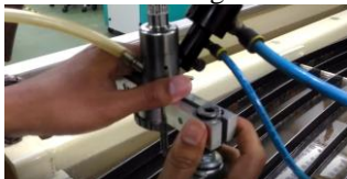
Fig. 11. Wheel and pillar place at the slot.
