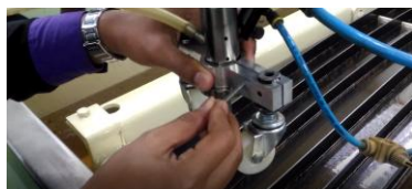
Fig 13. The clamp bar is tighten
