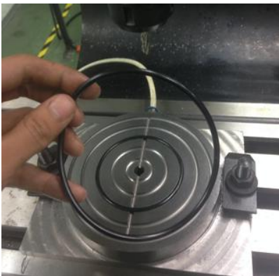
Fig. 8. Sealing cord place on top of the vacuum clamping
