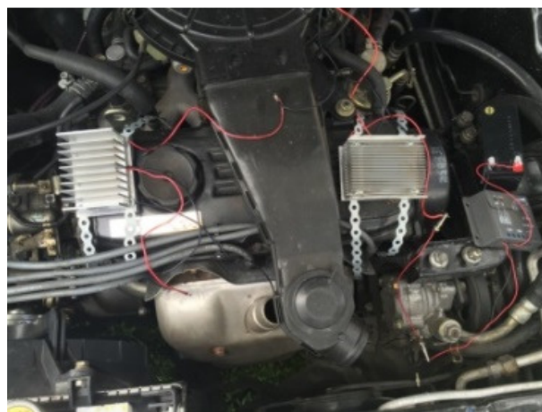
Fig. 3. Generating system on car engine system
