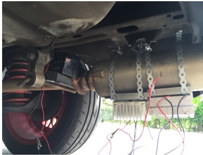
Fig. 4. Generating system on car exhaust system
