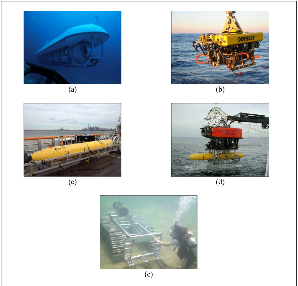
Figure 1.1: Types of Underwater Vehicles. (a) Human Operated Vehicle (HOV) adapted from Atlantis submarines.travel (2017). (b) Remotely Operated Vehicle (ROV) adapted from Shipwrecks: Artifacts & Treasure (2017). (c) Autonomous Underwater Vehicle (AUV) adapted from Exercise, G. (2018). (d) Hybrid Remotely Operated Vehicle (HROV) adapted from MBARI (2017). (e) Underwater Remotely Operated Crawler (ROC) Adapted from Florida Tech eCurrent (2017).
