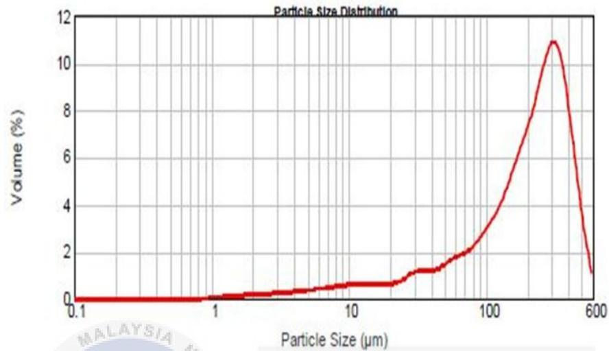
Figure 4.1 Particle size distribution of quarry dust
