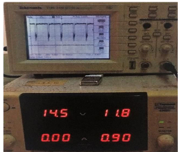
Figure-17. DC input voltage showing 11.8V and corresponding PWM waveform duty cycle (99%).
