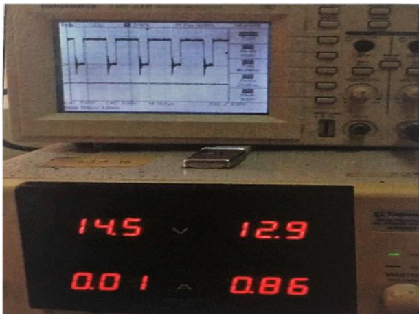
Figure-18. DC input voltage showing 12.9V and corresponding PWM waveform duty cycle (91%).
