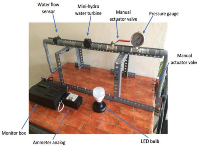
Figure 2: Residential piping designed system
