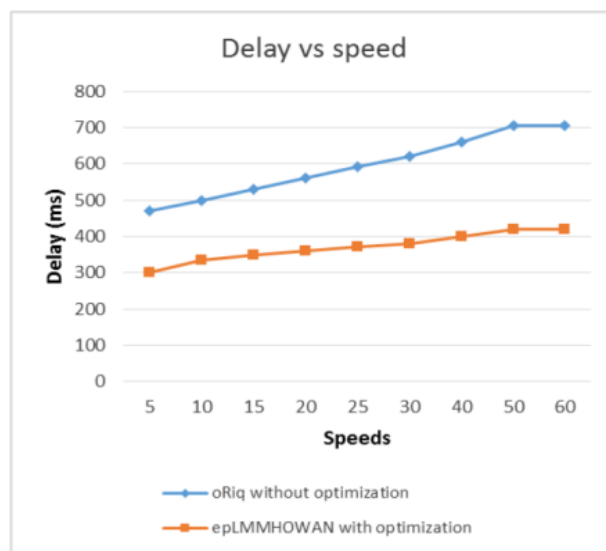
Fig. 5. Performance of end-to-end delay for varying speeds for both schemes of oRiG and SCMDR multi-parameter AODVUU routing before and after with self-configure mechanism based on Taguchi optimization
