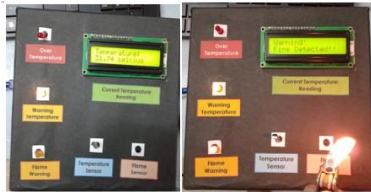
Figure 5. Temperature warning and fire detection
