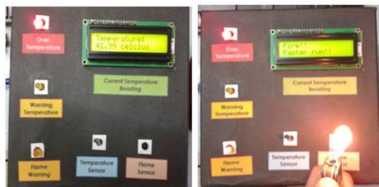
Figure 6. Over temperature and fire alert notification
