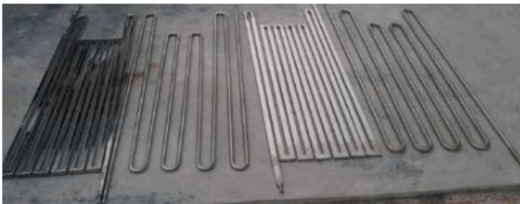
Fig. 46. Serpentine collector absorber of a PVT system: (from left), (A) square tube with 20 mm diameter, (B) round tube with 15 mm diameter, (C) rectangle tube hydraulic with 18.7 mm diameter, (D) round tube with 20 mm diameter [70]
