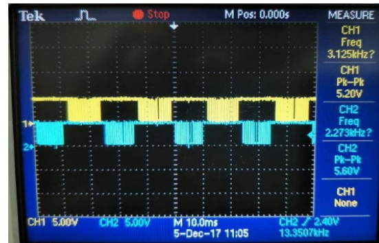
Figure 13. PWM Signal from TL494 for both low-side gate
