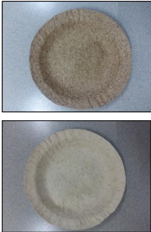
Figure 3:Biodegradable Plastic of Oil Palm Fiber (left) and Sugar Cane Fiber (right)
