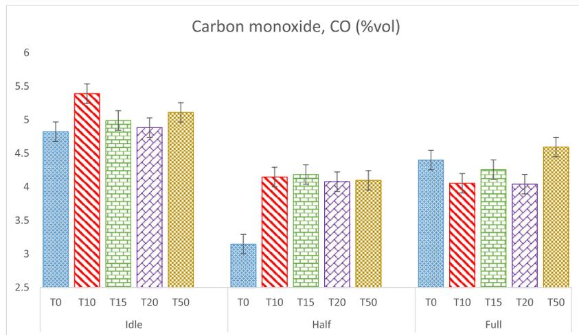
Fig. 4. Variation of CO emission as a function of engine speed for all lubricant-gasoline blends.
