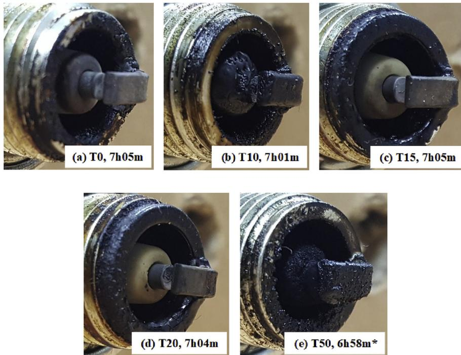
**Fig. 3.** Carbon deposition on spark plug at idling; (a) Fully-mineral T0 – wet deposit on circumference and dry deposit on electrodes, (b) T10 – wet deposit on circumference and dry deposit on electrodes, (c) T15 – dry deposit, (d) T20 – dry deposit, and (e) T50 – fouled, all wet deposits, \*calculated.
