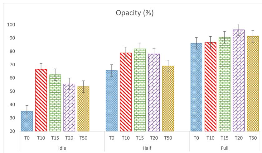
Fig. 7. Variation of opacity emissions as a function of engine speed for all lubricant-gasoline blends.
