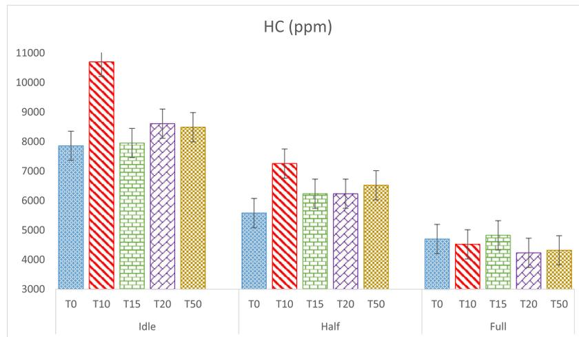
Fig. 6. Variation of HC emission as a function of engine speed for all lubricant-gasoline blends.
