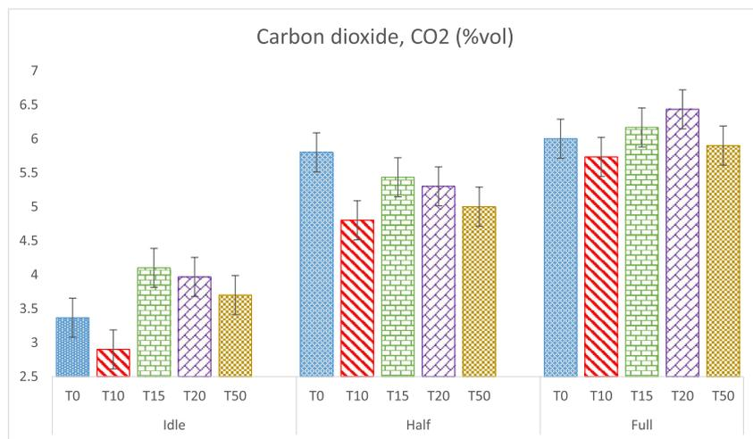
Fig. 5. Variation of CO<sub>2</sub> emission as a function of engine speed for all lubricant-gasoline blends.
