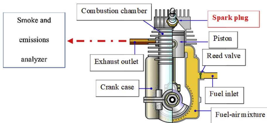
**Fig. 1.** Schematic diagram of the two-stroke engine.**Table 3**
