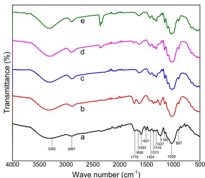
**Fig. 4 – Fourier transform infrared spectroscopy of (a) raw sugar palm fibre [54], (b) bleached fibre [54], (c) alkali-treated fibre [54], (d) refined fibre, and (e) sugar palm nanofibrillated cellulose.**
