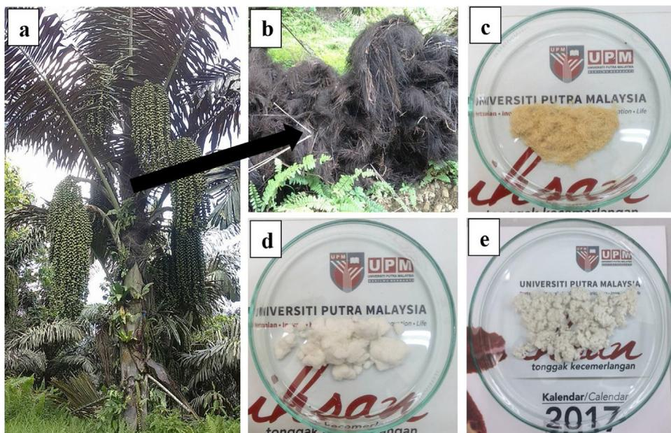
Fig. 1 – Photographs of (a) the sugar palm tree, (b) raw sugar palm fibres, (c) bleached fibres, (d) alkali-treated fibres, and (e) refined fibres.
