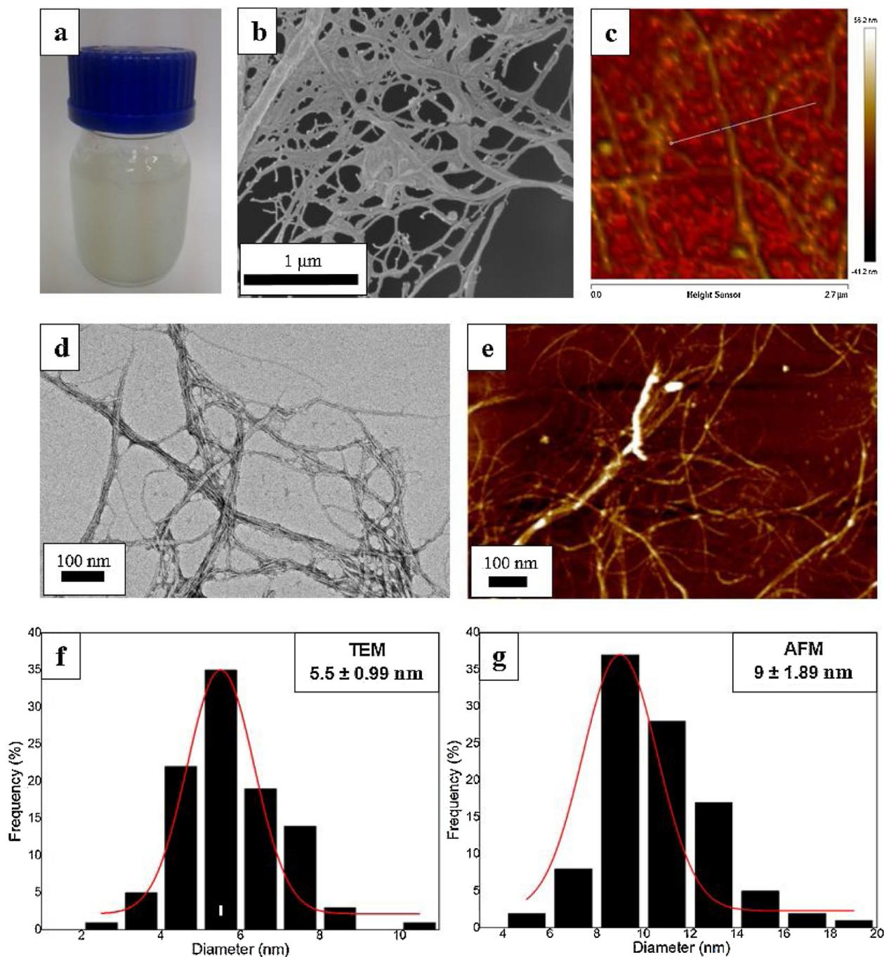
**Fig. 3 – (a) 2 wt% of nanocellulose suspension, (b) field emission scanning electron microscopy (FESEM) micrograph, (c) height dimension of NFCs by means of atomic force microscopy (AFM) nanograph, (d) transmission electron microscopy (TEM) nanograph, (e) atomic force microscopy (AFM) nanograph, and (f and g) their diameter histograms based on TEM and AFM nanograph.**
