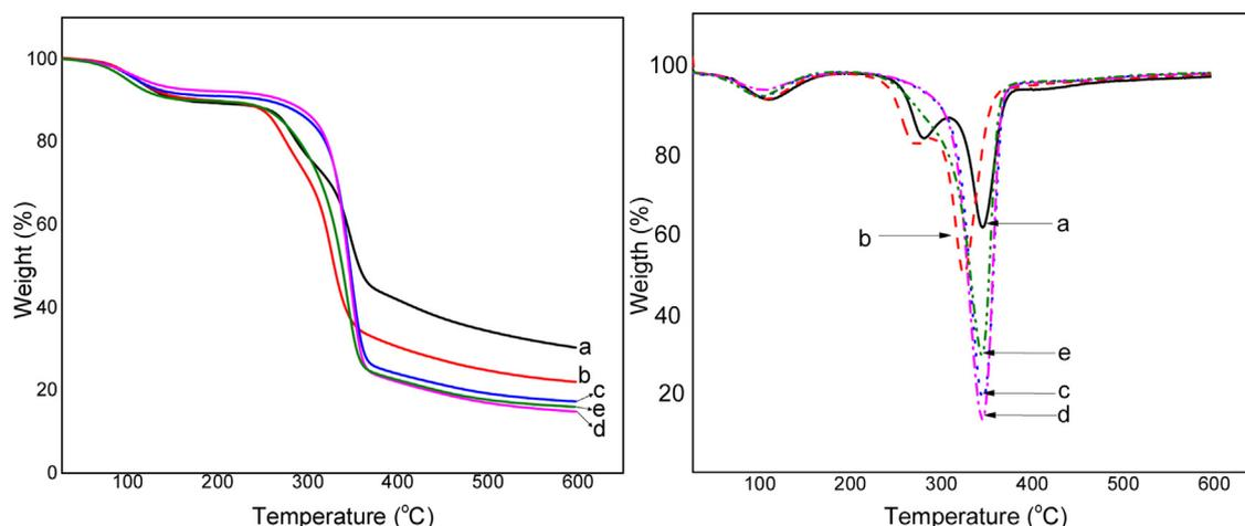
**Fig. 6 – (i) Thermogravimetry (TG) and (ii) derivative thermogravimetric (DTG) curves for (a) raw sugar palm fibres [54], (b) bleached fibres [54], (c) alkali-treated fibres [54], (d) refined fibre and (e) SPNFCs.**
