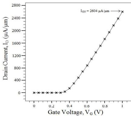
Figure 15. I-V curve at  $V_D = 0.5$  V for n-JLDGVM device with WF = 4.5 eV
