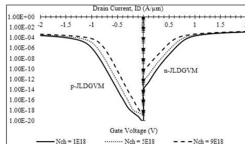
Figure 7. Graph of the subthreshold drain current (I<sub>D</sub>)-gate voltage (V<sub>G</sub>) at V<sub>D</sub> = 1.0 V with different concentration of channel doping
