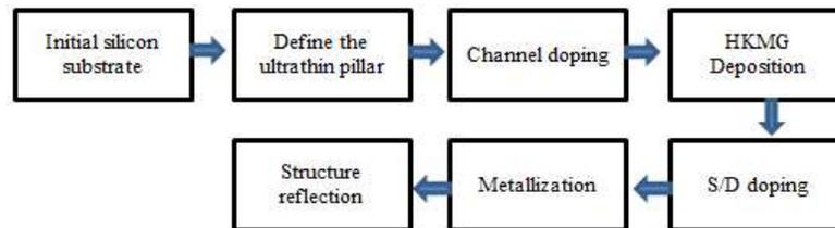
Figure 1. Simulated process flow for ultra-thin JLDGVM's design
