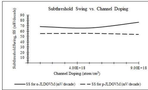
Figure 8. Subthreshold swing vs. channel doping
