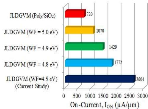
Figure 16. Benchmark of n-JLDGVM device with other junctionless vertical devices with multiple WF magnitude [18]
