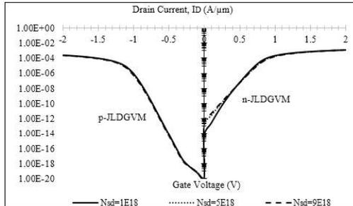
Figure 10. Graph of the subthreshold drain current ( $I_D$ )-gate voltage ( $V_G$ ) at  $V_D = 1.0$  V with different concentration of source/drain doping
