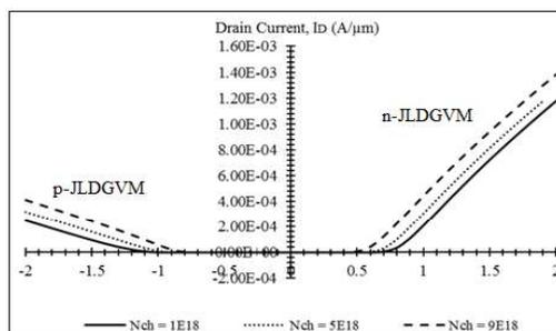
Figure 6. Graph of the drain current (I<sub>D</sub>)-gate voltage (V<sub>G</sub>) at V<sub>D</sub> = 1.0 V with different concentration of channel doping
