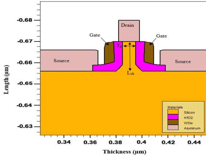
Figure 2. Cross section of the JLDGVM device
