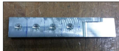
Figure-12. Finish drilling process.
