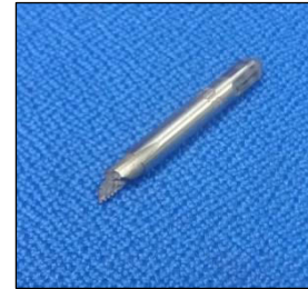
Figure-29. Broken tap.
