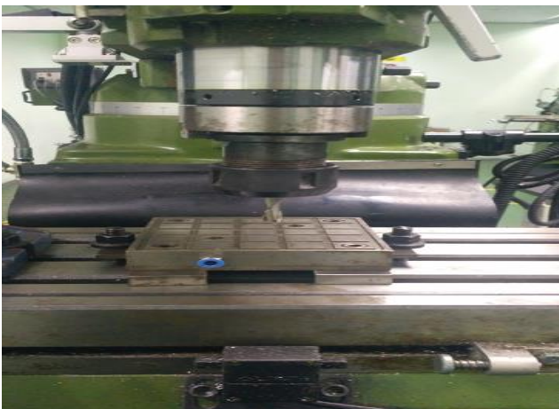
Figure-2.2. vacuum clamping at milling machine.
