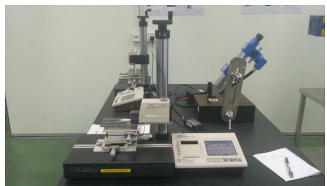
Figure-2.5. Surface roughness tester, SJ-410.
