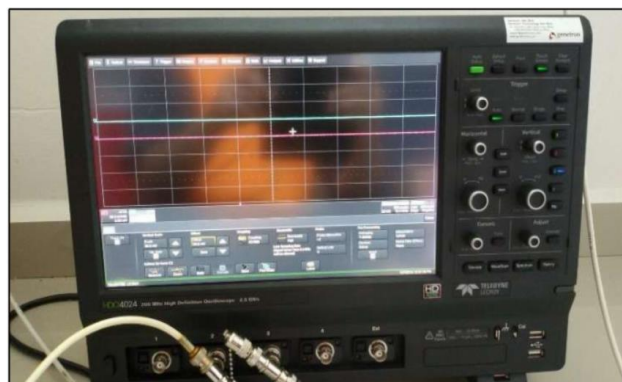
Fig. 4 - LeCroy HDO 4024 used to display the captured signal.
