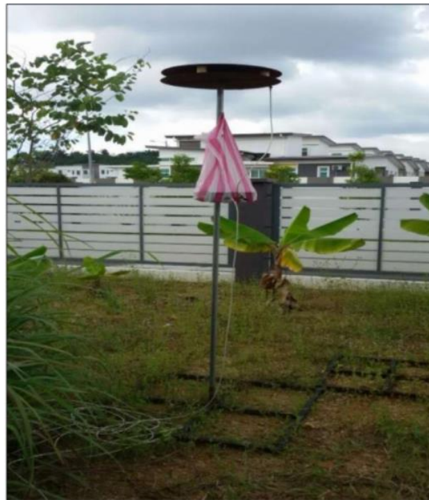
Fig. 3 - The antenna of parallel flat plate antenna was used in this study.
