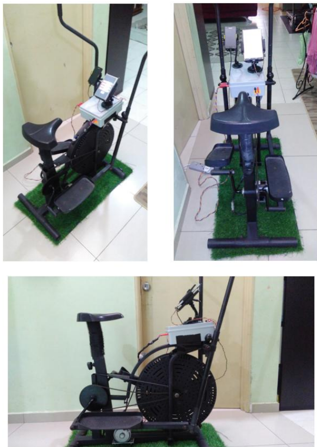
Fig. 10. The developed stationary cycling charger prototype.
