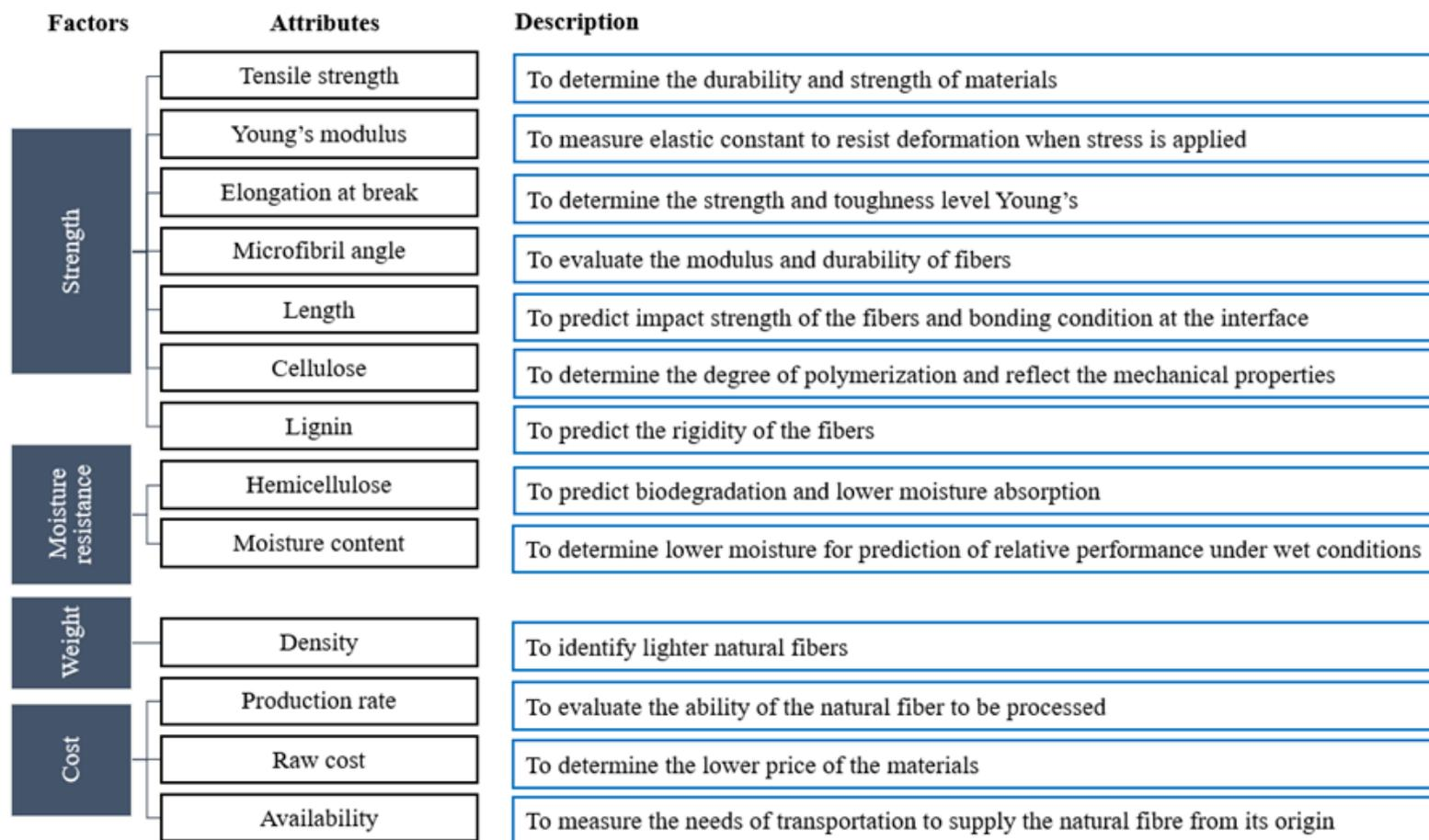
**Fig. 2.** Selection factors and attributes developed to find the most suitable natural fiber in biocomposites for food packaging application (Al-Oqla and Salit 2017; Mastura *et al.* 2017)
