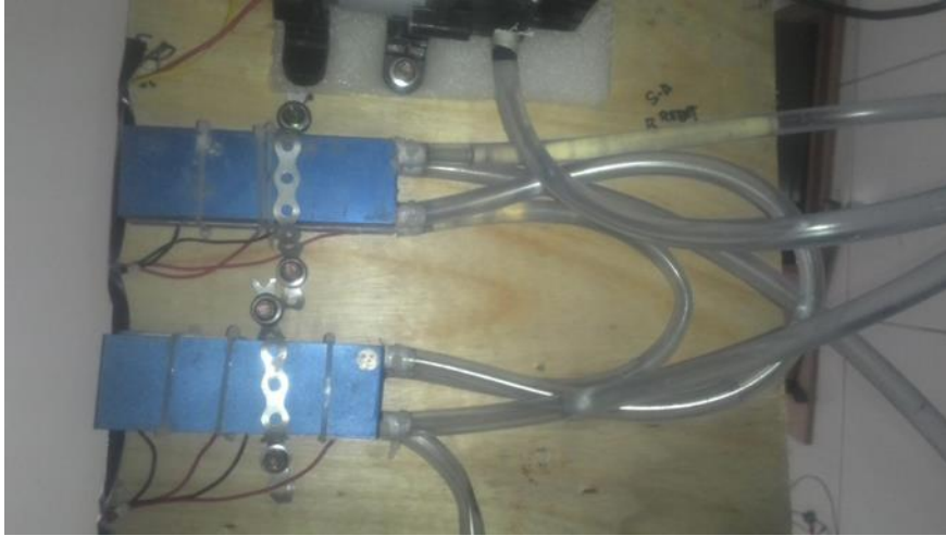
Fig. 3. Combination between Peltier and water block
