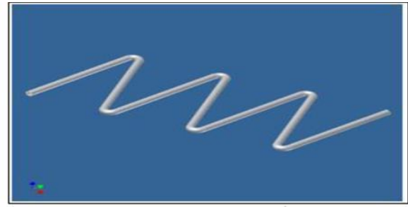
Fig. 37. Serpentine Flow Design of PVT [42]
