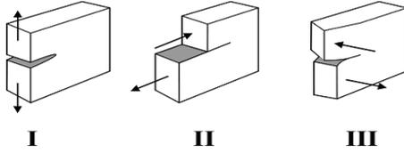
Figure 1. Three types of modes in fracture mechanics
