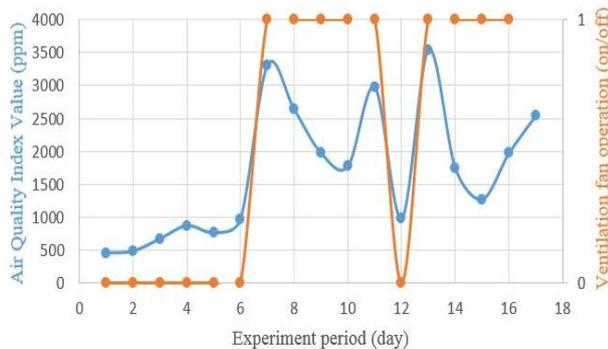
Fig. 10. Recorded AQI and Ventilation System Operation
