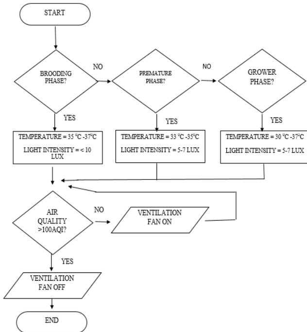
Fig. 2. Overall Project Operation Flowchart
