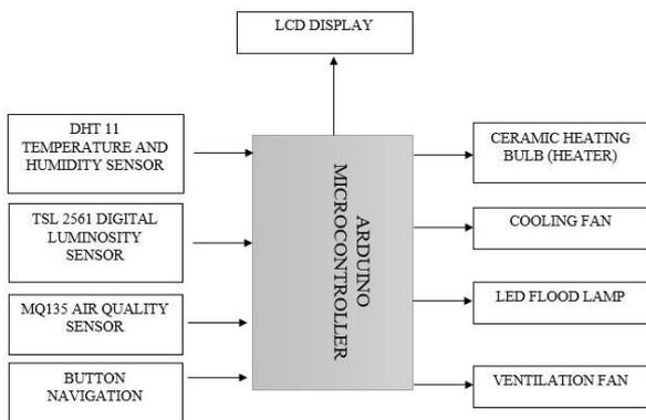
Fig. 1. Block diagram of Project IO declaration
