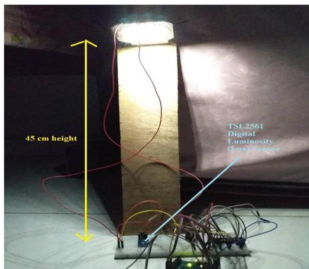
Fig. 7. PWM-LUX experiment setup
