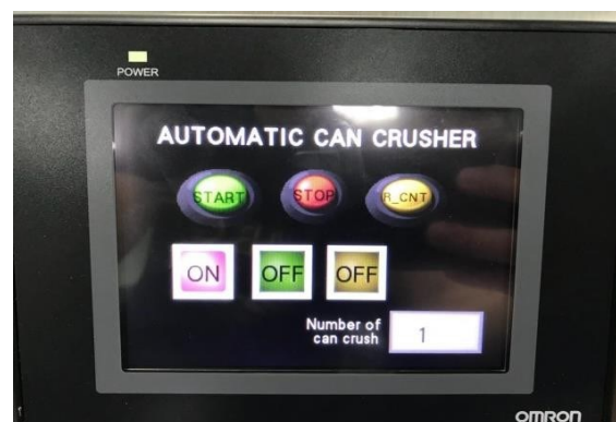
Figure 4. PLC - HMI interface using the NB-Designer software from OMRON shows how the Automatic Can Crusher complete its task with showing how many can it have crush
