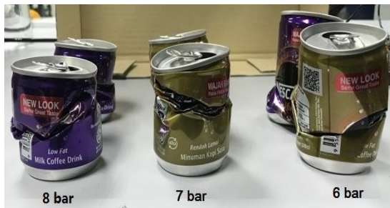
Figure 5. The desired size of Nescafe brand of the cans according to the pressure supply
