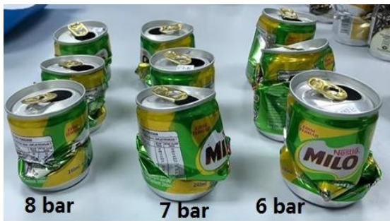
Figure 7. The desired size of the Milo brand of the cans according to the pressure supply
