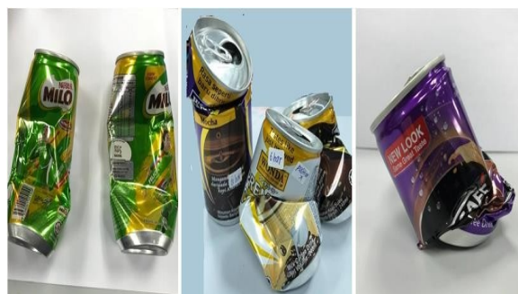
Figure 9. The sample of fail crushed can that could not be crushed perfectly
