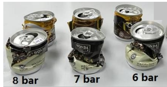
Figure 6. The desired size of Wonda brand of the cans according to the pressure supply
