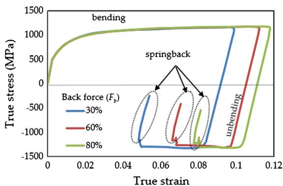
Fig. 16. Variation of stress value in the draw-bend test simulation [75].
