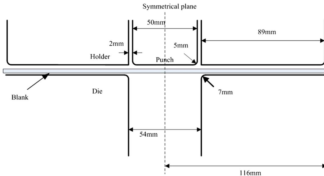
Fig. 7. Schematic view and dimension of 2D draw bend test equipment [42].
