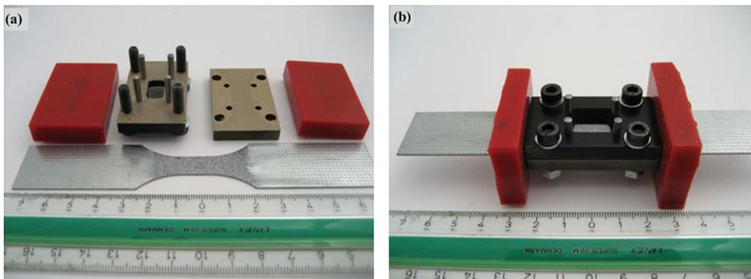
Fig. 10. Experimental apparatus for tension-compression test; (a) dismantled; (b) assembled [47].
