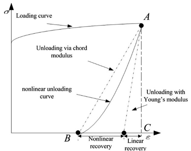
Fig. 13. Stress-strain curves for linear and nonlinear unloading [73].
