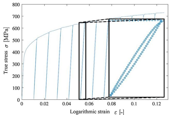
Fig. 14. Uniaxial cyclic test results [74].
