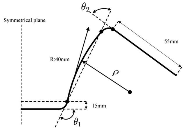
Fig. 8. Springback angle measurement [42].
