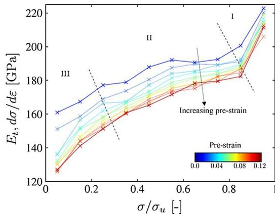
Fig. 15. Instantaneous tangent modulus vs normalized stress during unloading.
