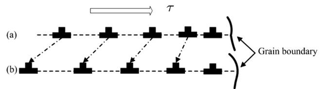
Fig. 12. Dislocation pile-up model: (a) loading; unloading [50].
