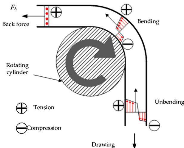
Fig. 17. Schematic of stress variation in the sheet metal blank [76].
