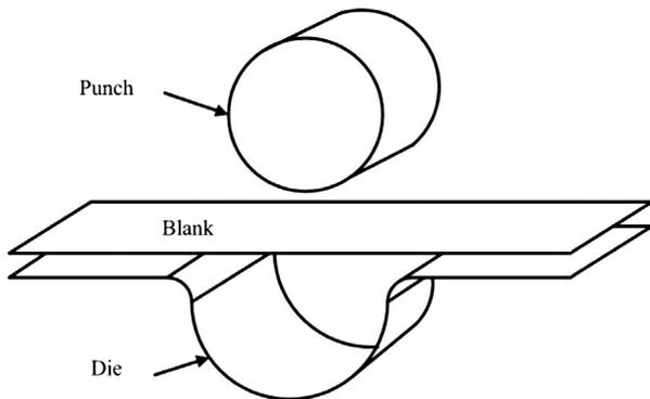
Fig. 4. Initial preparation of cylindrical tooling as suggested in Numisheet 2002 [19].
