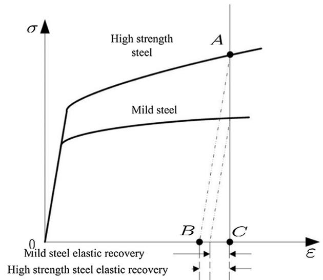
Fig. 1. Schematic of springback that is proportional to the stress level.
