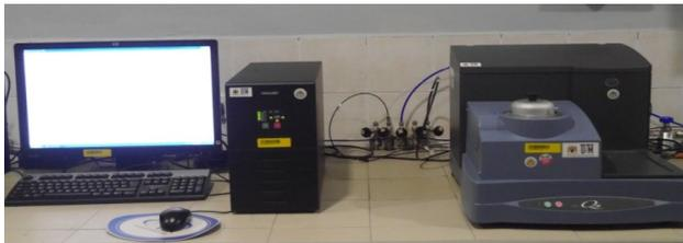
Figure 1: DSC Equipment of TA DSC Q20
