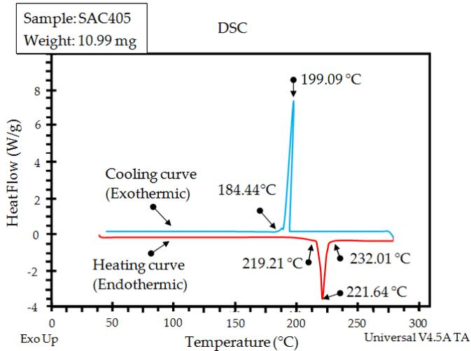
Figure 6: The heat flow of SAC 405 solder paste as a function of peak temperature
