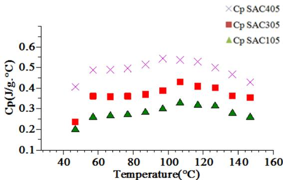
Figure 3: Experimental values for the specific heat capacity
