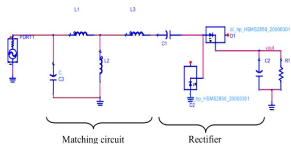
Figure-1. RF/DC Converter Schema.
