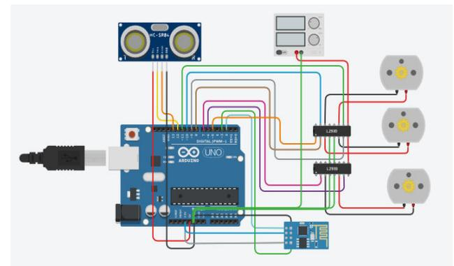
**Figure-2.** Connection of Multi-Controlled Floor Vacuum Cleaner.
