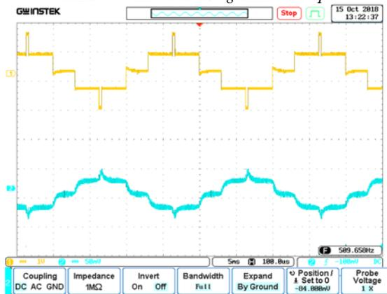
Fig 16. Non-optimisation of output voltage a and current waveform of a five-level CHB-MLIs with MI=0.55 using FFA technique.
