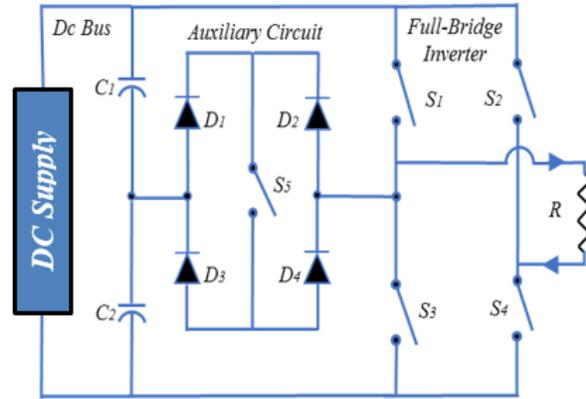
Fig 1: A Single-phase of a modified CHB-MLIs. for five levels.
