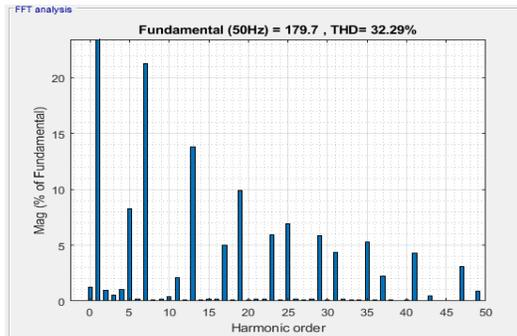
Fig 8. Non Optimization harmonic spectrum of single-phase output voltage waveform using FFA technique.
