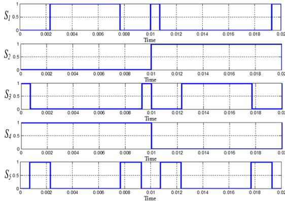
Fig 5. Switching pattern of a five-levels modified CHB-MLIs.
