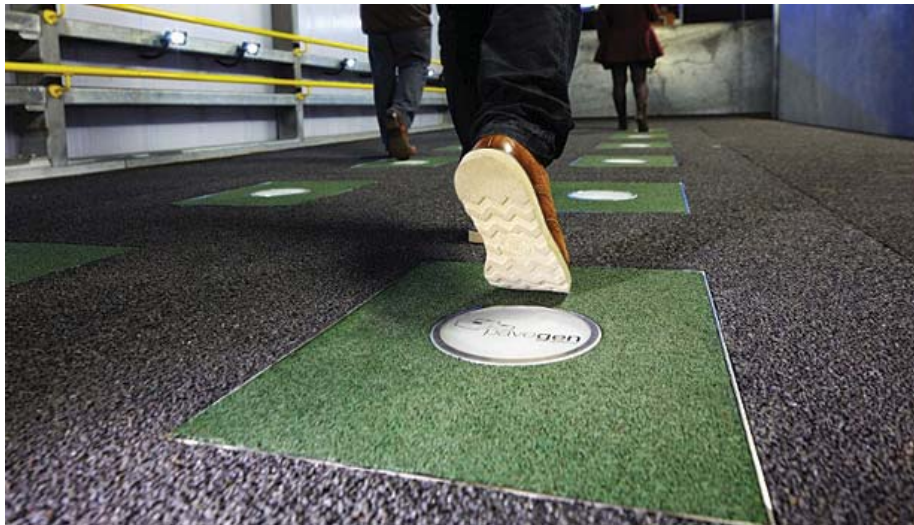
Figure 1.1 Tiles in floor to harvest energy from pressure from walking activities (Rosenfeld, 2014)
