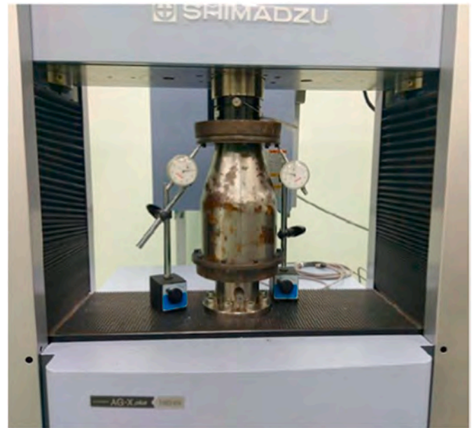
Fig. 4. Test set-up for cone-cylinder specimen under axial compression only.
