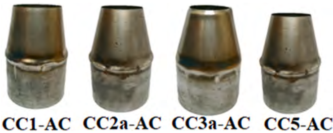
Fig. 7. Photograph of selected cone-cylinders specimens after testing.
