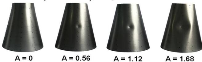
**Fig. 2. Typical photograph of conical specimens with different dimple amplitude.**
