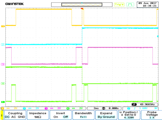
Figure-17. Switching pattern of a single-phase 13-levels modified CHB-MLIs for cell three comprising S_{11}, S_{12}, S_{13}, S_{14}, and S_{15} switches with MI=0.81 using PSO technique.
