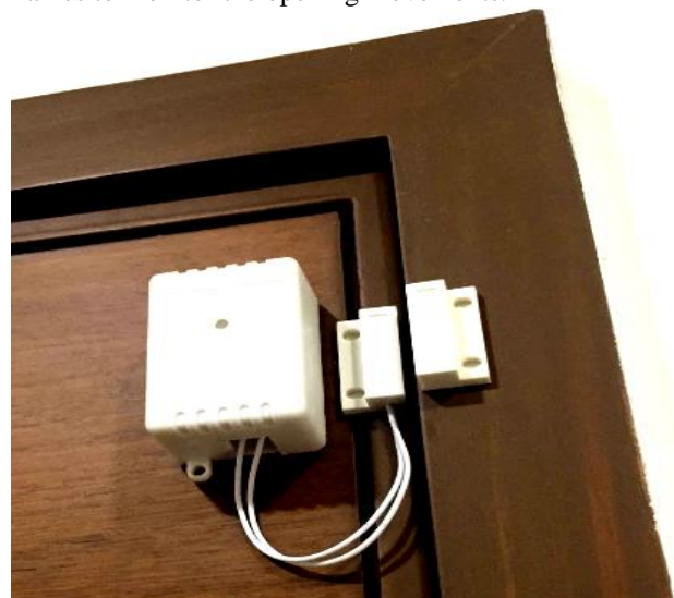
Figure-2. Magnetic based door - a door sensor with power sleep mode model: example [10].
