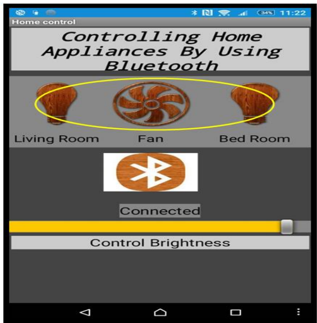
Figure-14. Living/Bed room appliances' control when their command Buttons are turned ON/OFF.
