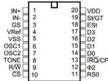
Figure 6: The IC8880 DTMF Decoder [17]
