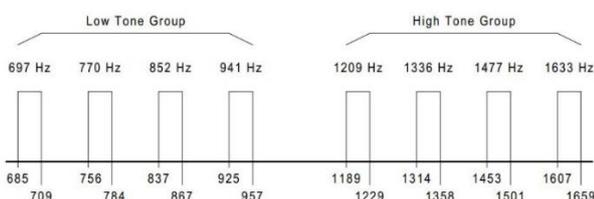
Figure 3: DTMF Frequency Spectrum [16]
