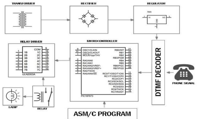
Figure 8: Block Diagram of Home Appliances Controller
