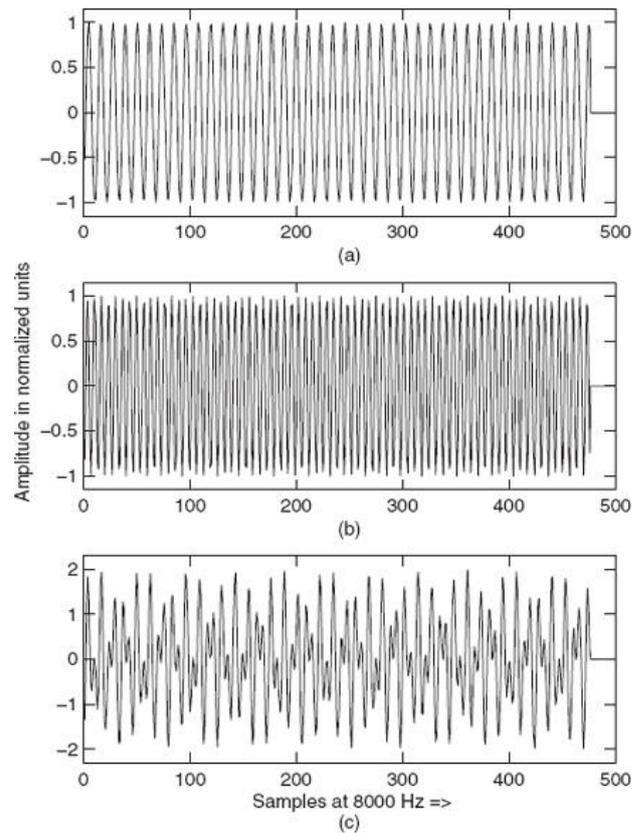
Figure 4: Digit-1 tone generation example for 320 samples, 40ms. (a) Row tone at 697Hz at unity amplitude. (b) Column tone at 1209 Hz at unity amplitude. (c) Combined tones for digit-1 [16].
