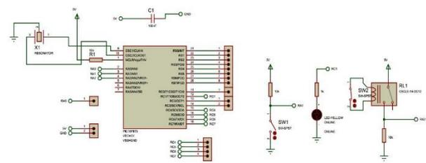
Figure 11: Central Control Unit Circuit
