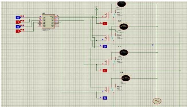
Figure 15: Simulating relay with AC load
