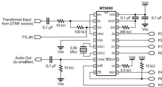
Figure 7: The IC8880 Single End Input Connection [17]
