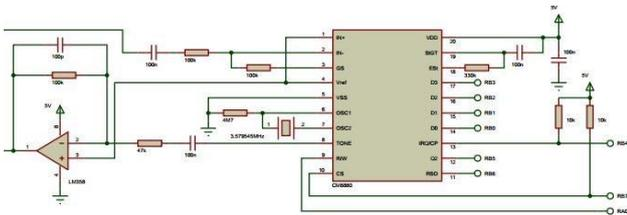
Figure 10: DTMF Communication Unit Circuit
