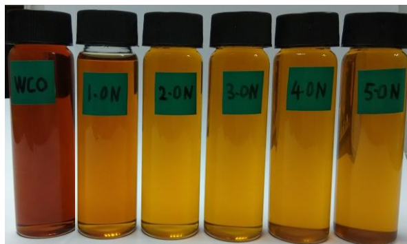
Fig. 3. Colour of the WCO and neutralized WCO samples (normality of caustic soda: 1.0, 2.0, 3.0, 4.0, and 5.0 N)
