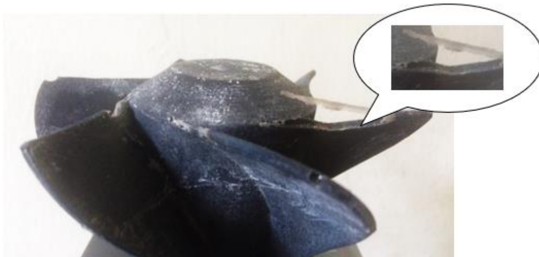
Fig. 6. Expected defect due to lack of venting system
