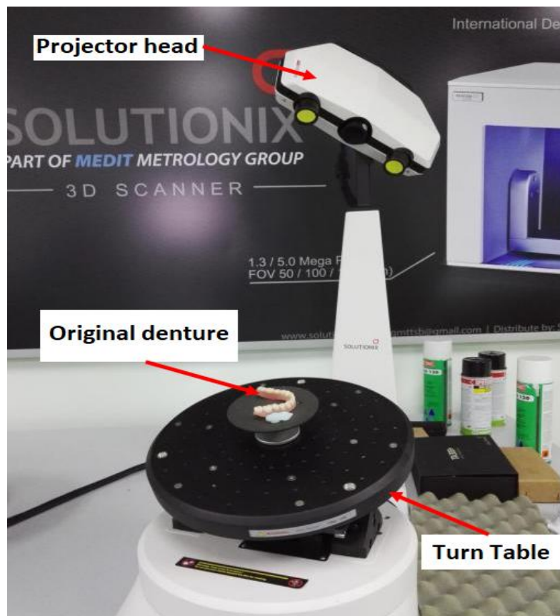
Fig. 3. Rexscan 3D scanner built with blue light technology.
