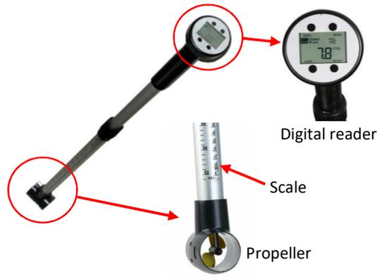
**Fig. 2.** Flow velocity probe for flow velocity measurement
