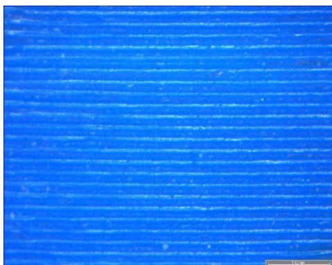
Figure 5. Surface roughness view of the best RaV sample 3 with parameter value; At: 30 °C, Lt: 0.178 mm and Pa: 67.5°
