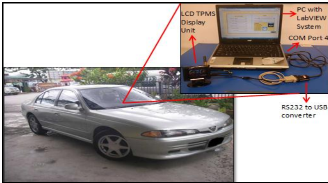
Fig. 8: Tyre pressure deflation test setup on a vehicle
