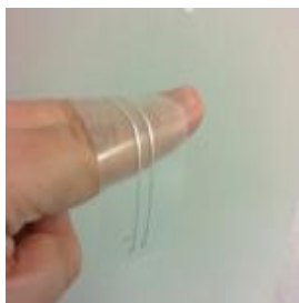
Figure 1. Stretchable Conductive Ink based on screen-printed silver paste [3].
