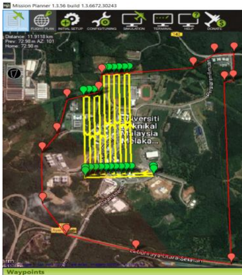
Figure 8: Waypoints of the third flight plan covering 53.93 Hectare of the study area
