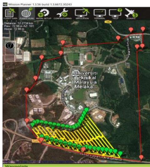
Figure 10: Waypoints for the fifth flight plan covering 49.15 Hectare of the study area
