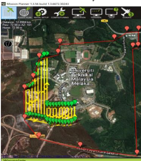
Figure 9: Waypoints for the fourth flight plan covering 51.59 Hectare of the study area
