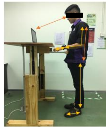
Fig. 12: The standing posture of Respondent B using the new ergonomics computer table
