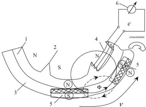
**Figure-1.** Scheme of the magnetic separator performance measurement method by magnetic product.
