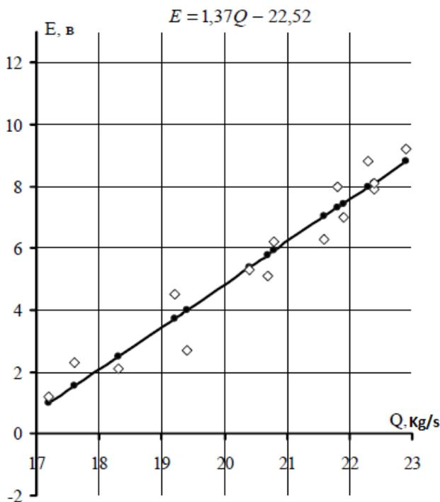
**Figure-3.** Regression equation of the electromotive force (E) of the performance of the separator for the magnetic iron Calculation Results: Regression Equation  $E = 1,37Q - 22,52$  ; coefficient of determination  $r^2 = 0,94$  ; correlation coefficient  $r = 0,97$  .
