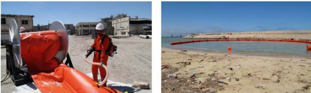
Figure 2.0: Inflatable Light Boom (ILB), a curtain boom type (Muizis, 2013)
