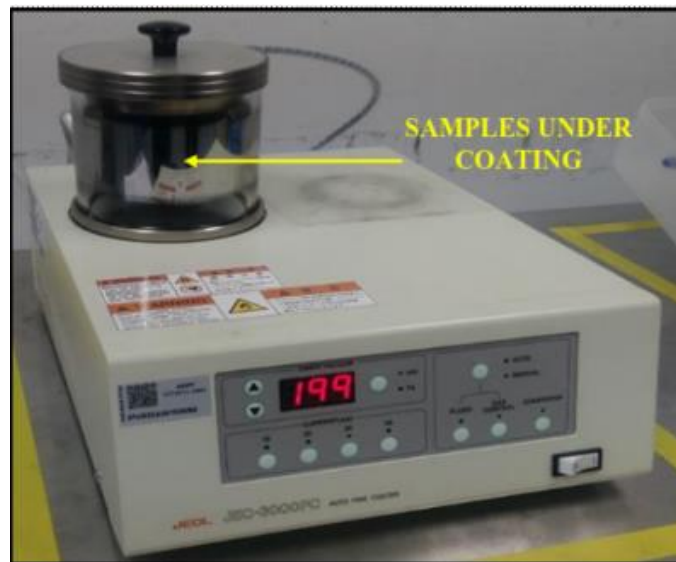
Figure 4: Coating of Samples with Gold Material to Create a Conductive Layer
