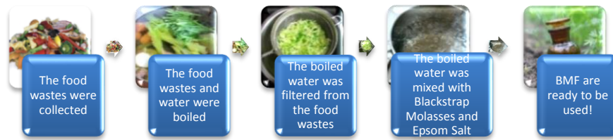
Fig. 1. Process of making fertilizer from the food wastes.
