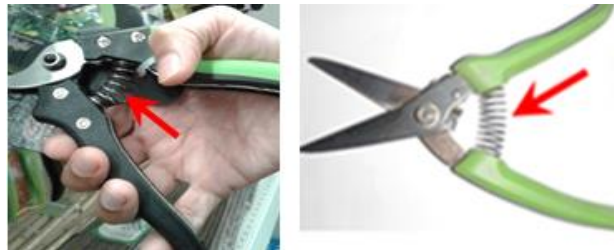
Fig. 7 - Spring is used in operating a pruner
