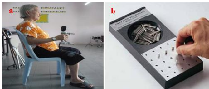
Fig. 12 - Grip strength measurement (a) [110]. Dexterity test using grooved peg-board (b) (Lafayette Instrument, USA)
