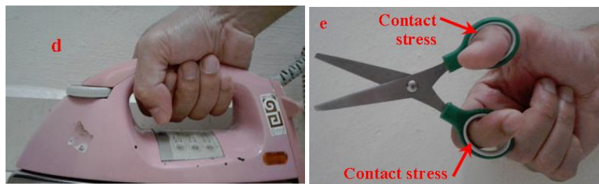
Fig. 11 – Good clearance around the handle (d) and contact stress due to insufficient clearance (e)
