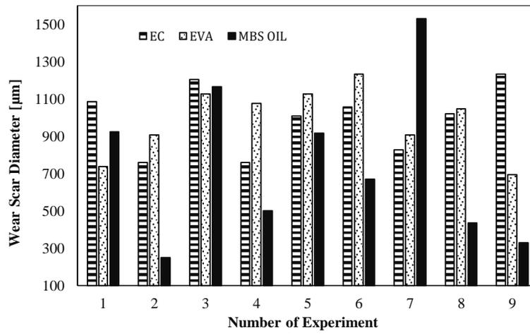
Figure 4: Variation Value of Wear Scar Diameter of MBS Oil with the presence of EC and EVA at Different Concentration.
