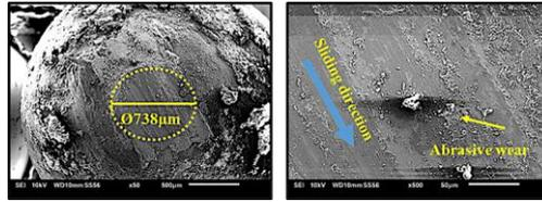
Figure 4.33a: Worm Surface and Wear Mechanism on the Hemispherical Pin with Addition of 0.5 % w/w of EVA at 27 °C and Load of 60 N (Experiment 1) Observed using SEM.
