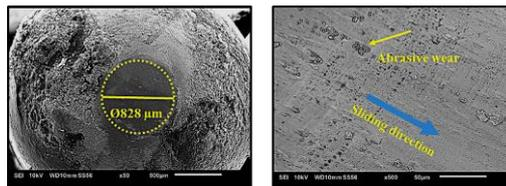
Figure 4.32a: Worn Surface and Wear Mechanism on the Hemispherical Pin with Addition of 4.0% w/w of EC at 27 °C and Load of 100 N (Experiment 7) Observed using SEM.
