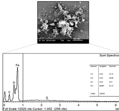
Figure 4.34b: EDX Images of Worn Surface of the Hemispherical Pin with Addition of 0.5% w/w of EVA at of 27 °C and Load of 100 N (Experiment 3) Observed using SEM.
