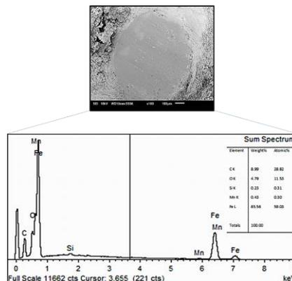
Figure 4.32b: SEM-EDX Images of Worn Surface of the Hemispherical Pin with Addition of 4.0% w/w of EC at 27 °C and load of 100 N (Experiment 7) Observed using SEM.
