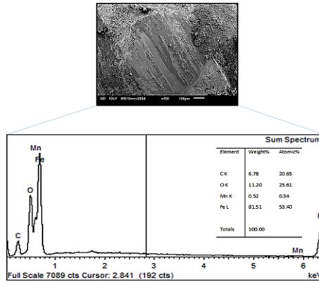
Figure 4.33b: SEM-EDX Images of Worn Surface of the Hemispherical Pin with Addition of 0.5 % w/w of EVA at 27 °C and Load of 60 N (Experiment 1) Observed using SEM.
