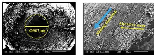
Figure 4.35a: Worm Surface and Wear Mechanism on the Hemispherical Pin with Addition of 4.0% w/w of EVA at 27 °C and Load of 100 N (Experiment 7) Observed using SEM.
