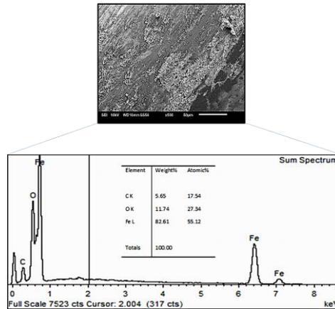
Figure 4.35b: EDX Images of Worn Surface of the Hemispherical Pin with Addition of 4.0% w/w of EVA at 27 °C and Load of 100 N (Experiment 7) Observed using SEM.
