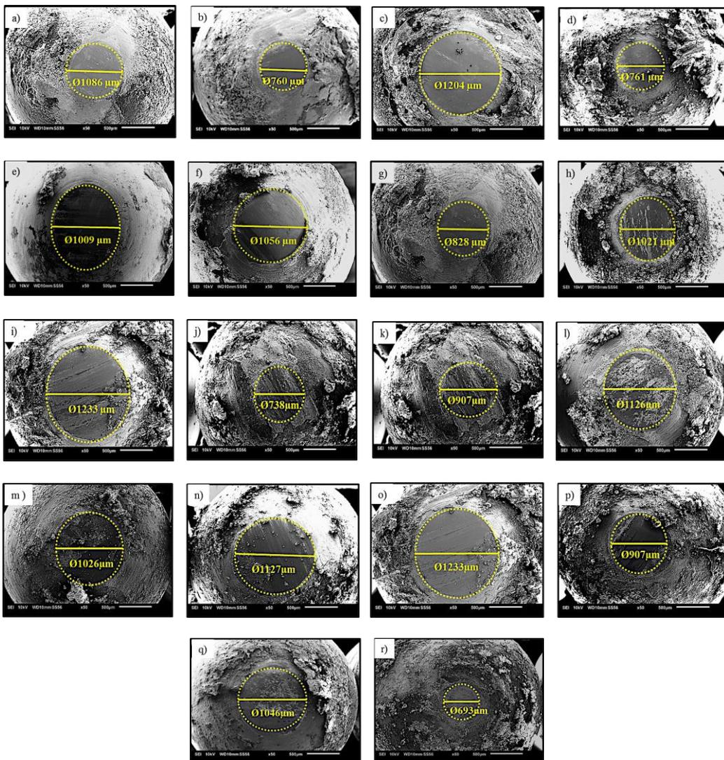
Figure 5: SEM Micrograph of Worn Surface of Hemisphere Pin at the Presence of EC (a-i) and EVA (j-r) at Different Concentration.
