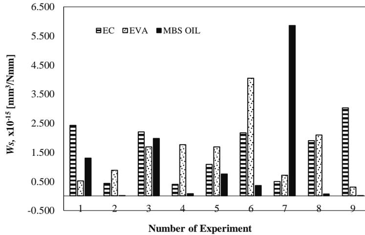
Figure 6: Variation Value of Wear Rate,  $W_s$  of MBS Oil with the Presence of EC and EVA at Different Concentration.
