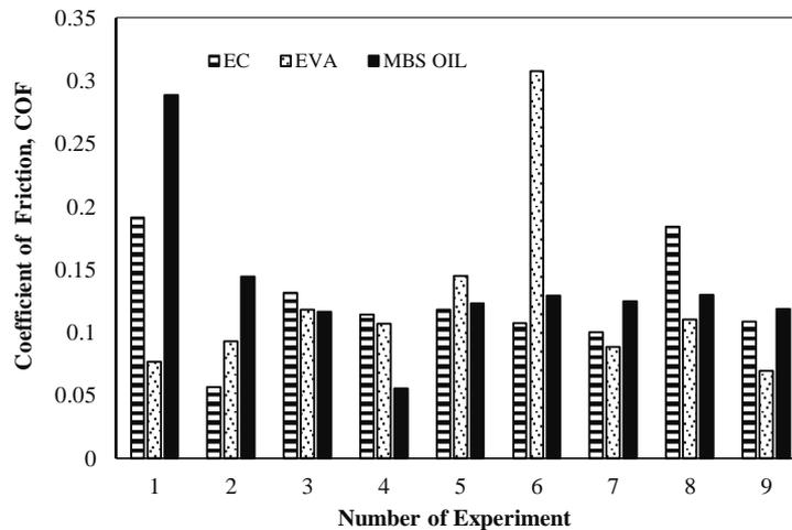
Figure 3: Variation of COF Value of MBS Oil with the Presence of EC and EVA at Different Concentration
