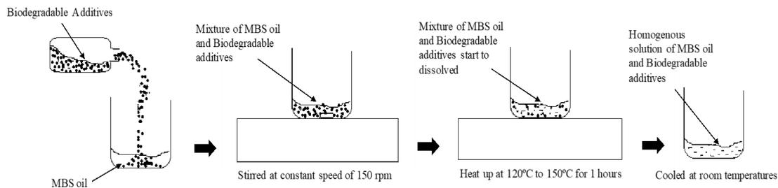
**Figure 1:** Schematic diagram of preparation of MBS oil with biodegradable additives
