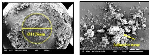
Figure 4.34a: Worm Surface and Wear Mechanism on the Hemispherical Pin with 0.5% w/w of EVA at of 27 °C and Load of 100 N (Experiment 3) Observed using SEM.
