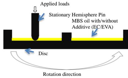
**Figure 2:** Schematic diagram of pin on disc.
